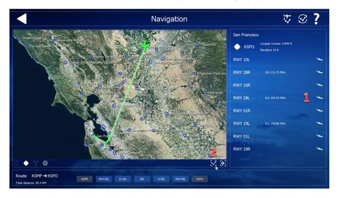
We don't want to turn immediately to the right after take off, so let's go on with an additional VOR. VOR means *Very High Frequency Omnidirectional Radio Range*. A VOR ground station sends out signals, which are used for standard air navigation for both commercial and general aviation.
