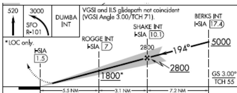
This is the glide path to the runway. To intercept the glide path, our flight level in a distance of 17.4 nm is at or below 5000 ft.
