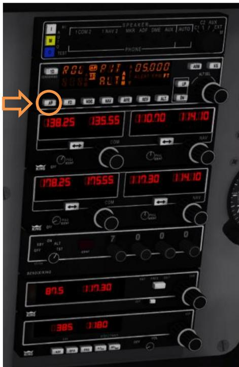
Adjust average power, level your aircraft and press the key A to activate the Autopilot (alternatively press AP at the control panel).
